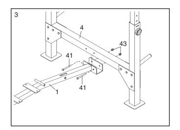
Attach the Bench Frame (1) to the Crossbar (4) with two M10 x 85mm Bolts (41) and two M10 Nylon Locknuts (43).
